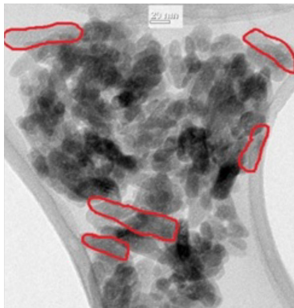
Figure 2. Micrographs of the synthesized hydroxyapatite nanoparticle sample.
