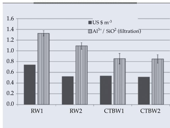
Figure 6. Relation produced aluminium-removed silica and unitary cost per cubic meter.
