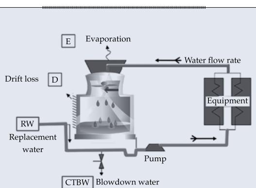
Figure 1. Mass balance of water for a cooling tower.
