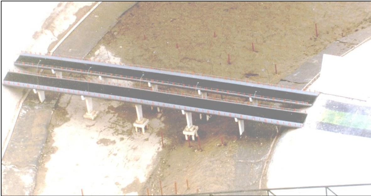
Figure 2. Physical model of Cáceres bridge piers (Universidad de Piura, 2001).
