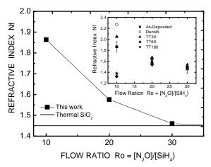
**Figure 1.** Refractive index as a function of Ro for as-deposited films, a comparison with thermal  $SiO_2$  is done. The inset shows the Refractive index as a function of Ro for different annealing times.
