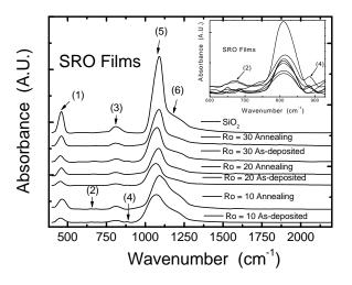
**Figure 2.** FTIR Absorption Spectra of the SRO films of Ro = 10, 20 and 30 after different annealing, and absorption spectra of thermal  $SiO_2$ . The capital letters (R), (B) and (S) mean Rocking, Bending and Stretching vibration modes.
