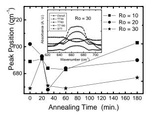
**Figure 3.** Peak position of the vibration modes at  $660-680 \text{ cm}^{-1}$  as a function of the annealing time for SRO films, the inset shows the absorption peak for Ro = 30.
