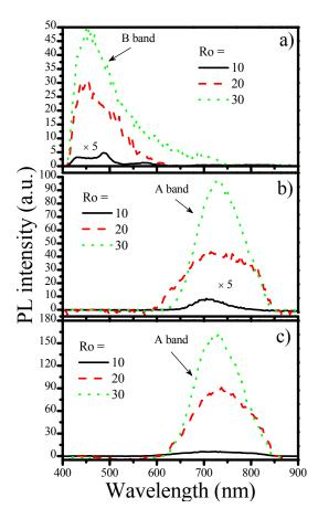
**Figure 4.** PL spectra of SRO with Ro = 10, 20 and 30 and a) asdeposited, b) densified at 1000 °C for 30 min, and c) thermally annealed at 1100 °C.
