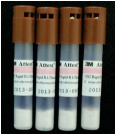
Figure 1. Rapid lecture biological indicators for autoclave use.
