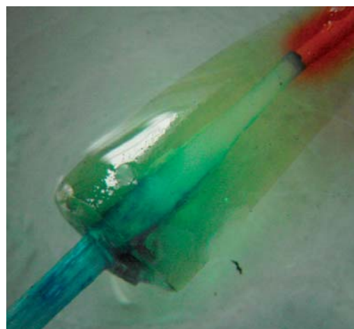
Figure 1. RelyX system endodontic post (3M ESPE dental products) exhibiting microleakage through the dentin-post inter-phase.
