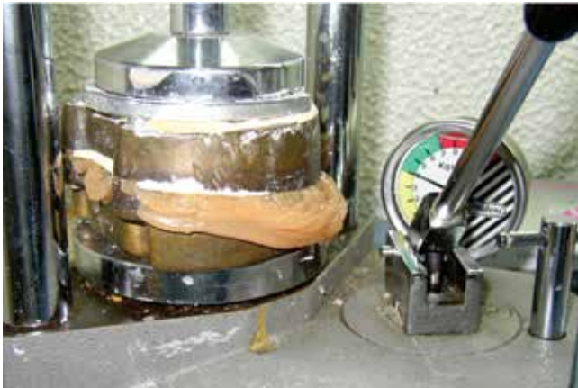
Figure 28. Muffle pressing with hydraulic press.
