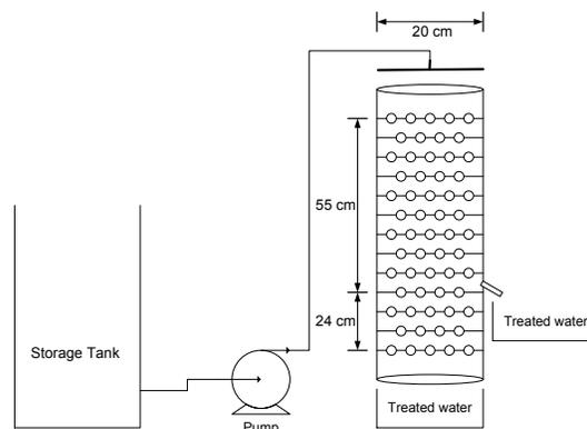
Fig. 1. Diagram of the experimental set up.
