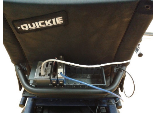
Figure 18. NI Compact-RIO installed for the real-time system.
