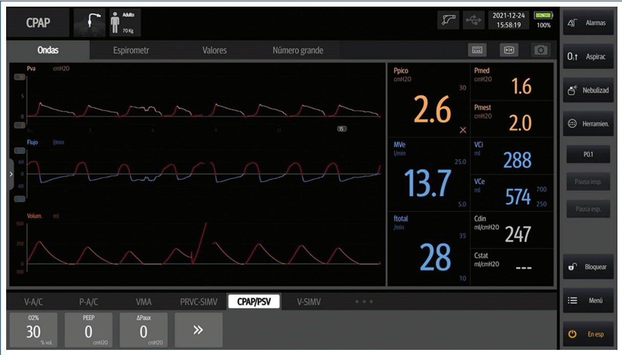
Figure 3. SBT performed with pressure support 0 cmH 2 O and positive end-expiratory pressure 0 cmH 2 O.
