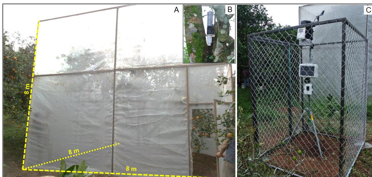
Figure 1. HLB-asymptomatic qPCR CLAs positive Valencia Citrus sinensis / C. aurantium orange tree confinement. A. Metal confinement structure (8 x 8 x 8 m) with aphid-proof netting. The structures included a key-restricted access door; B. HOBO U23 Pro V2 sensor for temperature (°C) and relative humidity (RH), programmed to take measurements at 30-minute intervals withing the confinement area; C. Davis Vantage weather station for measuring complementary climate variables such as precipitation, wind speed and direction, evapotranspiration, etc.
