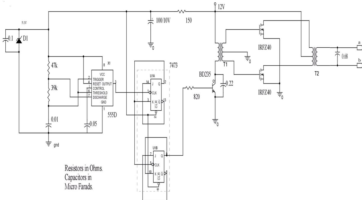
FIGURE 6. Electronic circuit of the DC/AC inverter.
