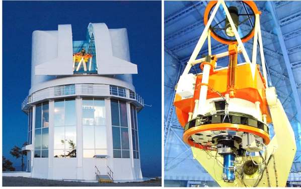
Fig. 1. The left image shows the main building of the Guillermo Haro Astrophysical Observatory (OAGH) in Cananea, Sonora, México. The 2.12 m telescope is shown on the right image with CANICA attached as the back-end instrument. The telescope is a Ritchey-Chrétien design with an equatorial fork mount.
