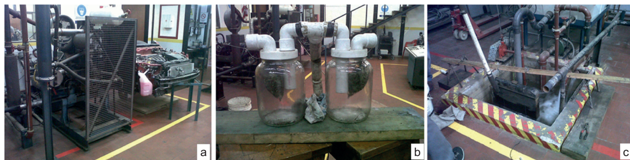
Fig. 3. Exposure chambers and experimental equipment. (a) Diesel engine; (b) glass chambers with biomonitors bags; (c) cooling system.
