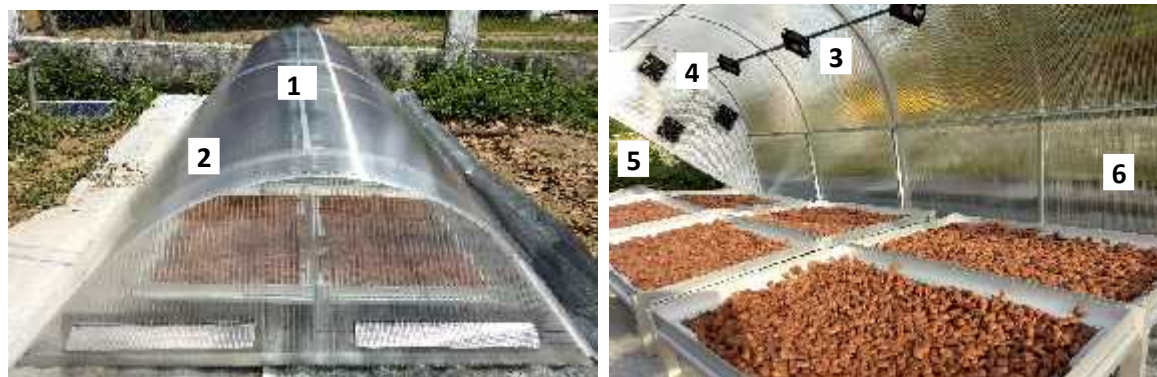
Figure 2. Main parts of the polycarbonate tunnel type solar dryer. 1) polycarbonate cover with UV protection; 2) windows that allow air to enter; 3) fans to homogenize the internal heat; 4) exhaust fans; 5) carriage holder; and 6 trays.
