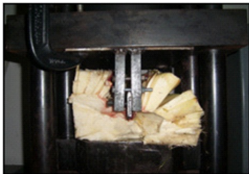
Figura 10. Muestra de agave fracturada. Figure 10. Fractured agave sampling.
