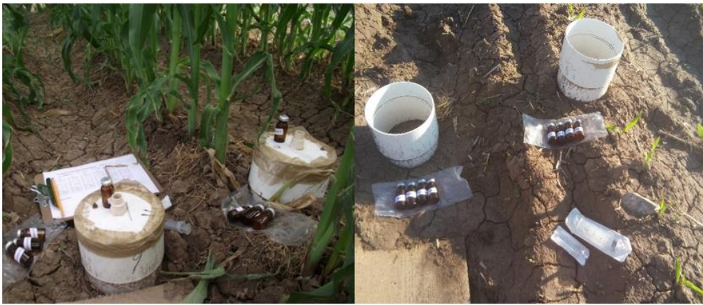
Figure 1. Placement of the static flux chambers at the ridge (B) and at the bottom (F) of the furrow with the necessary material for gas sampling.
