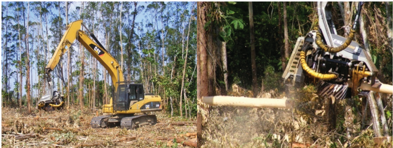
Figura 1. Cosechadora forestal, cabezal Kesla adaptado a la excavadora Caterpillar, Huimanguillo, Tabasco. Figure 1. Forest harvester, Kesla harvester head adapted to Caterpillar excavator, Huimanguillo, Tabasco.
