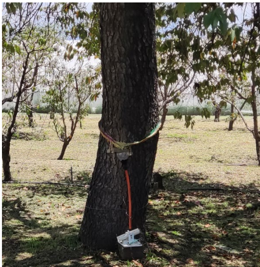
Figure 5. Arrangement used to measure stemflow in Prunus capuli Cav.
