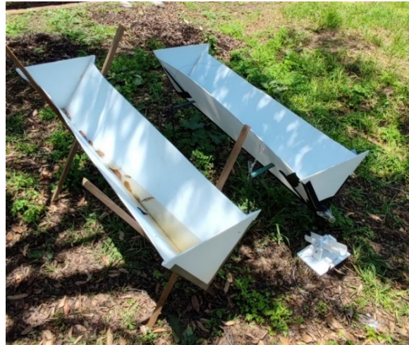
Figure 6. Arrangement of gutters used to estimate canopy flow.
