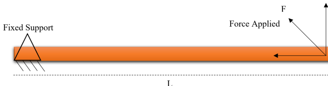
Figure 3. Diagram of the cantilever beam deflection experiment.
