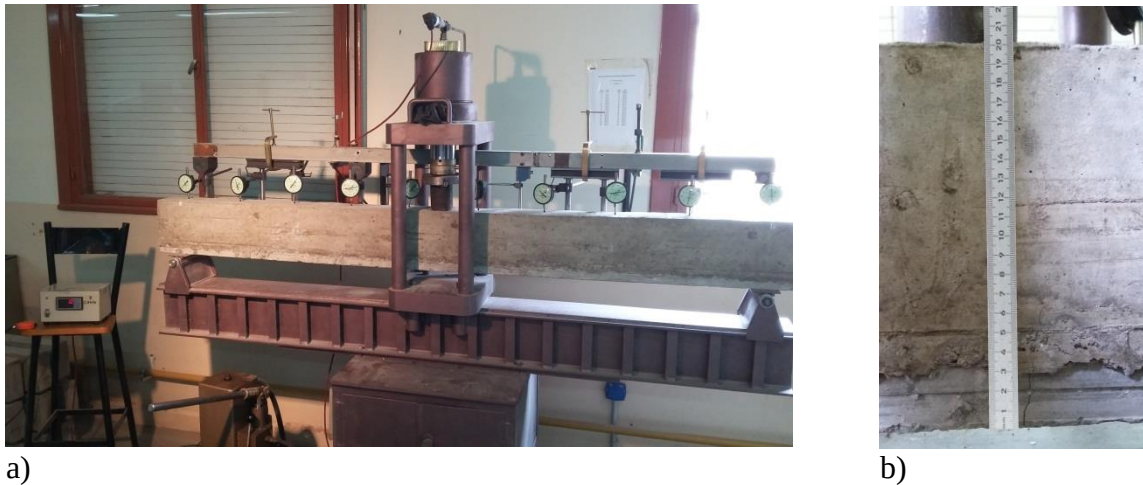
Figure 2. Test on Beam 01. a) General view. b) Measurement of the crack.
