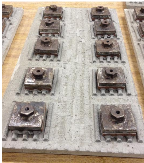
Figure 4. Metallic pieces attached on the ceramic tiles adhered to the substrate-pattern.
