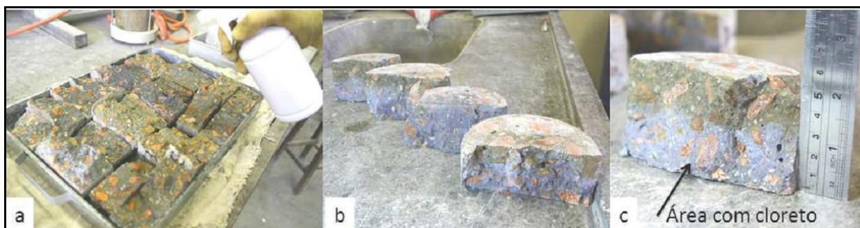
Figure 1. a) Spray silver nitrate solution; b) Comparison of the specimens; c) Measurement of the chloride penetration depth (MARCONDES, 2012)
