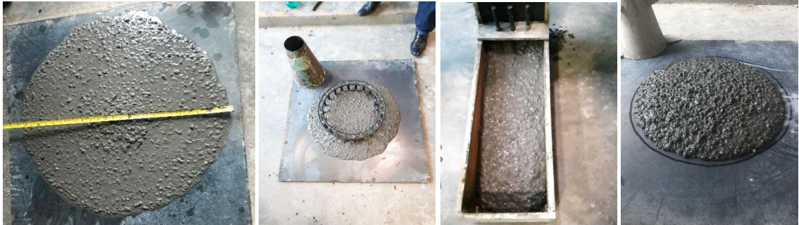
Figure 3. Mixtures on fresh state characterization for the evaluation of the elemental parameters of workability for a CAC.
