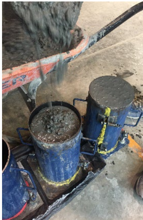
Figure 1. Filling of cylinders with self-compacting concrete.
