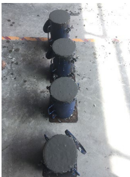
Figure 2. Preparation of the cylinders for the essay.
