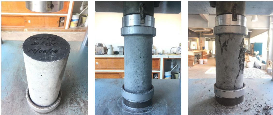
Figure 4. Test for the compression resistance sequence.
