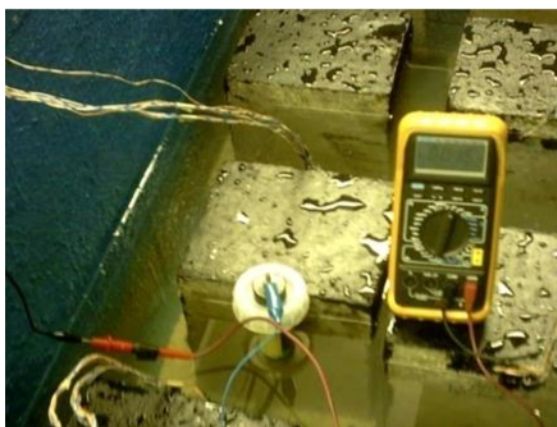
Figure 4. Monitoring with multimeter and Cu/CuSO 4 reference electrode.
