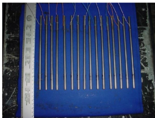
Figure 3. Type 304 Stainless Steel cathodes with copper wire connection, fastened with an industrial hose.
