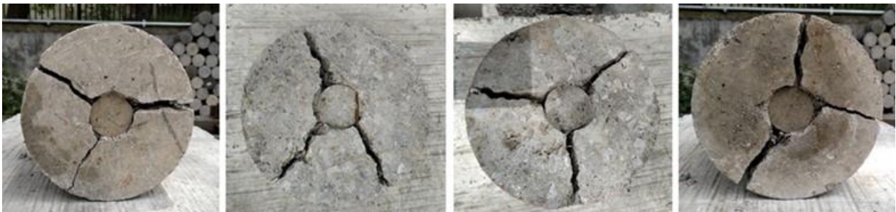
Figure 12. Cylinders typical failure mode, Barcelona Test.
