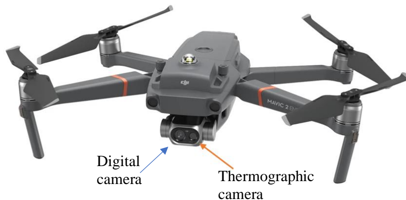
Figure 3. UAV with a thermographic camera attached to a digital camera (Topdrone, 2020).
