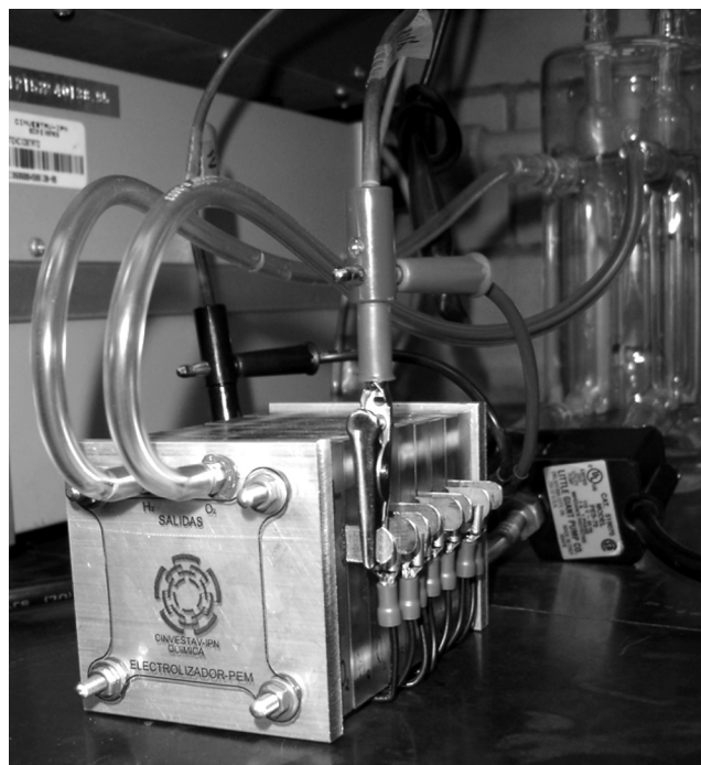
Fig. 1. The solid polymer electrolyte (SPE) electrolyzer designed and manufactured for the removable energy demonstration.
