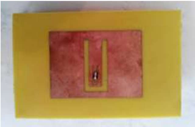
Fig. 13. Fabricated structure of the patch.
