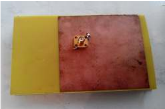
Fig. 14. Fabricated structure of ground.
