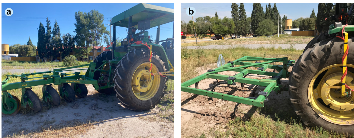
Figure 3. a) Disk plow and b) chisel plow used in the trials.
