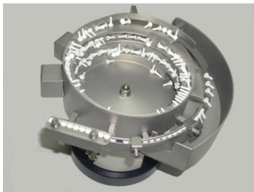
Fig.25. Vibratory feeder with orientation of elements
