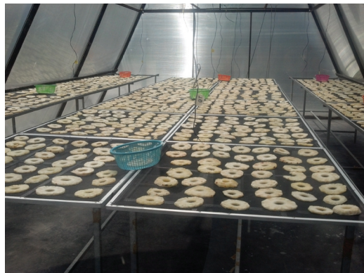
Figure 2. Pineapple slices uniformly laid out on trays for greenhouse solar drying operations
