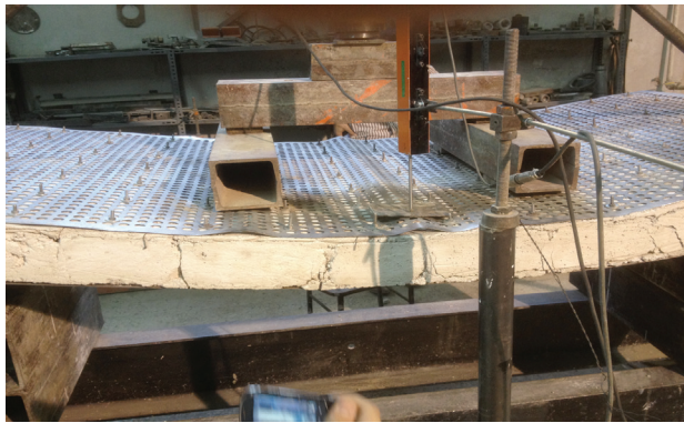
Figure 5. Buckling of the compression plate
