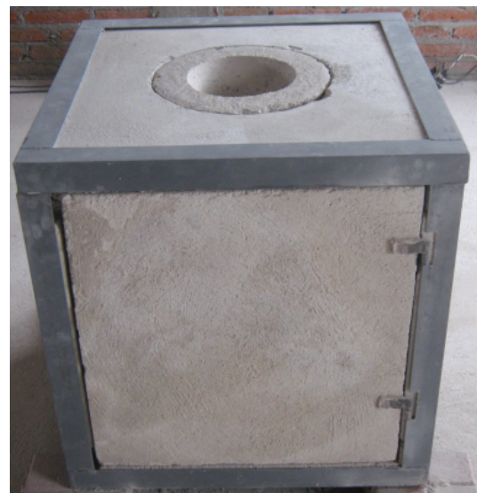
Figure 6. Photograph of the firing chamber
