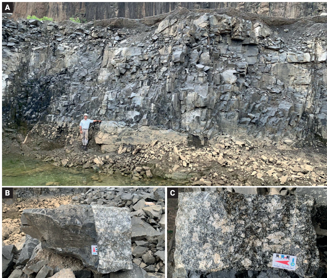
Figure 3. Diabase block in contact with gray porphyritic granite (left), detail of porphyritic granite with dark gray matrix composed of biotite and quartz (right), mining front with contact between strongly fractured columnar diabase (above) and porphyritic granite with not very expressive horizontal fractures (below).
