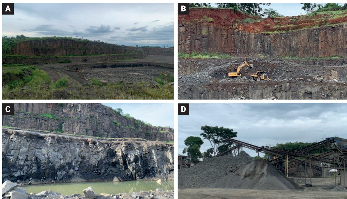
Figure 1. Main compartments of the study area. A) Panoramic view of the open pit mine. B) Bottom of pit with diabase saturated in water. C) Loading and transportation of dismantled rock, with soil and columnar diabase in the background. D) Crushing process and stacking the ore for sale.
