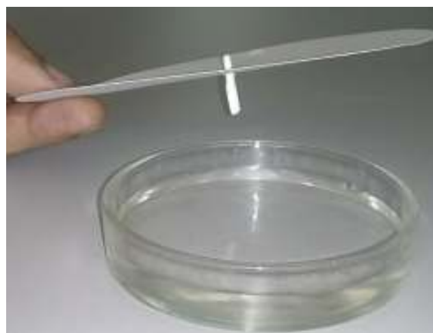
Figure 1 The impregnation process of the filters with AgNO_3 .
