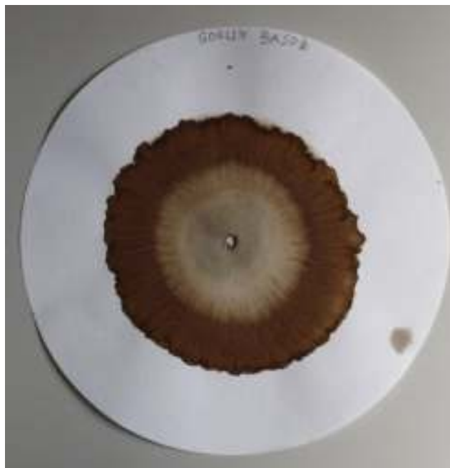
Figure 6 The chromatogram of the soil from a holm-oak wood.
