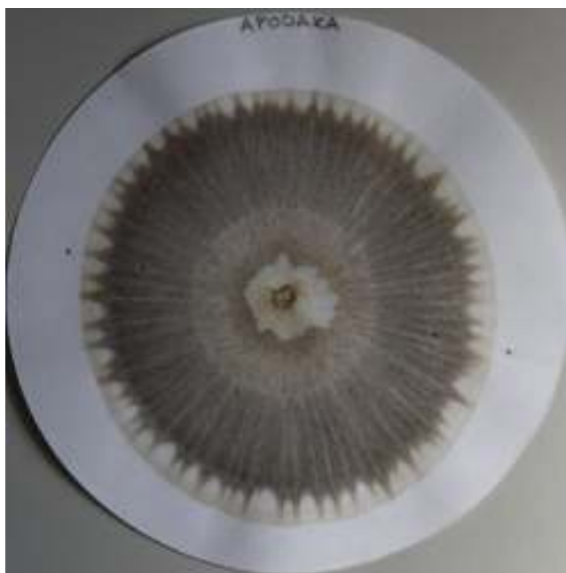
Figure 5 The chromatogram of the sample from a cereal crop field.
