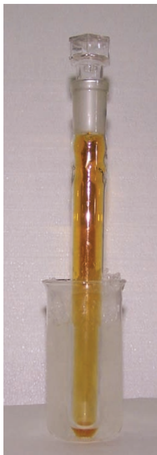
Figure 2. Test-tube with \text{N}_2\text{O}_4 (in equilibrium with \text{NO}_2 ) placed in ice bath.
