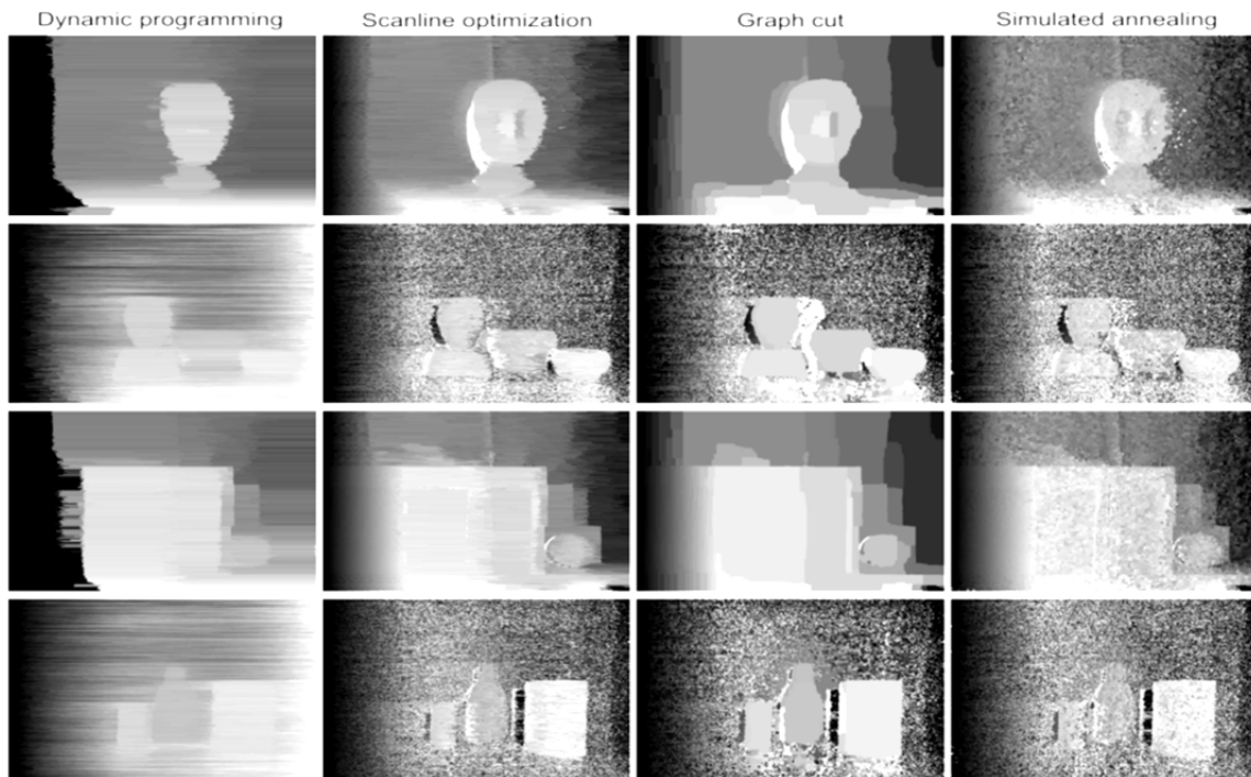
Fig. 14. Results using different optimization methods. From top to bottom, disparity maps obtained from angular ratio images in scenarios Edy, Fps, Gift, and Bot are shown. From left to right, the following optimization approaches are presented: dynamic programming, scan line optimization, graph cut, and simulated annealing
