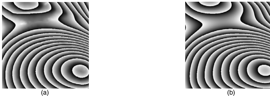
Fig. 3. (a) Gray level codification of a wrapped phase map recovered from a holographic interferogram. (b) Unwrapped phase map (shown wrapped for comparison purposes) obtained with the proposed method
