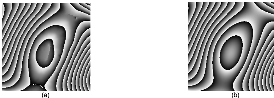
Fig. 4. (a) Gray level codification of a wrapped phase map recovered from an interferogram. (b) Unwrapped phase map (shown wrapped for comparison purposes) obtained with the proposed method
