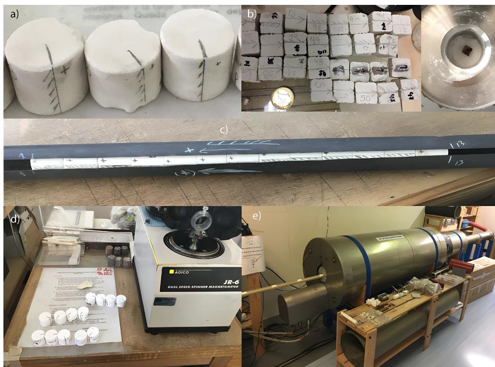
Figure 3 a) Sample assembly in salt cylinders (2.5 cm in diameter); b) Mounting of samples in a high-temperature-resistant diamagnetic plaster matrix; c) Sample holder used for heating samples embedded in salt; d) JR-6 spin magnetometer at IGF-UNAM; e) 2G cryogenic magnetometer at CEREGE-CNRS.
