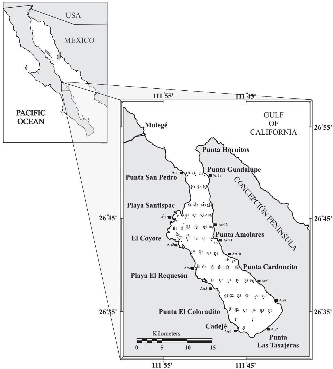
Figure 1. Location of Bahía Concepción, Baja California Sur, showing sample stations. Sediments were collected with a Petit Ponar grab sampler from a boat along east-west transects (dots) and by hand at the arroyos (squares).
