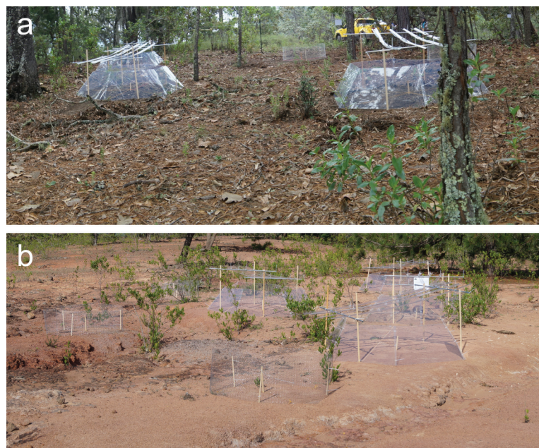
Figure 1. Experimental units used to assess effects of climate change on the recruitment of Quercus eduardii in the forest site (a) and in the clearing (b). The plates show control plots fenced with wire mesh and the climate change simulation plots (CCS plots). Each CCS plot consisted in an open-top chamber of transparent acrylic and a rainout shelter of transparent polycarbonate.
