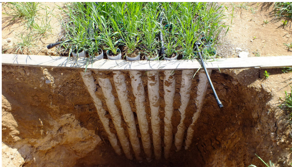
Figure 1. PVC tubes were replaced to above 200 cm depth in soil under field environmental conditions
