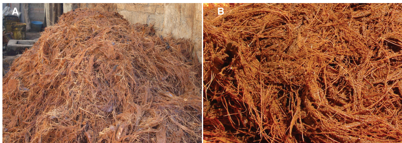
Figure 1. A) Cooked Agave angustifolia bagasse piled up in a traditional “ Palenque .” B) Close-up of bagasse fibers piled up.
