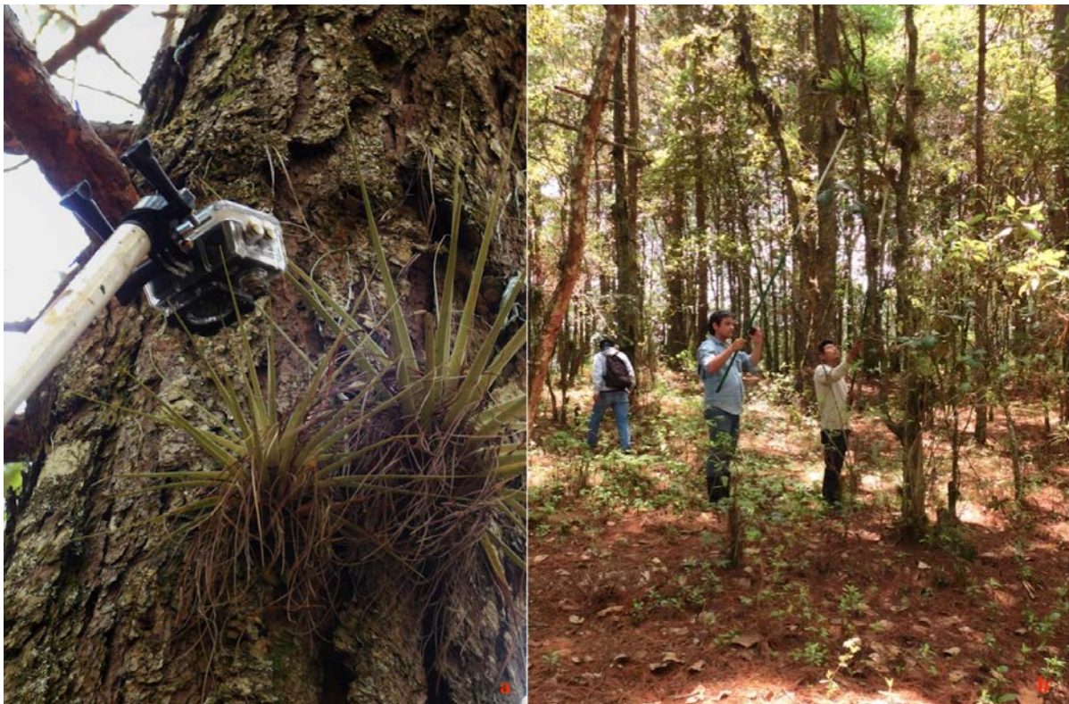
Figure 3. Spy eye technique, used for direct observation of Abronia lythrochila . a) wireless camera (GoPro HERO5 Black) mounted to an extendible pole; b) technique used, including two people.
