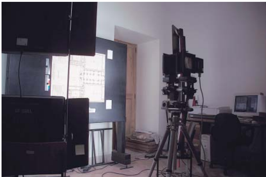
3. Scanning original drawings in high resolution at the Bibliotheca Hertziana in Rome. The whole digitalization-system is mobile and was already used for scan-campaigns in Milan and Berlin.
