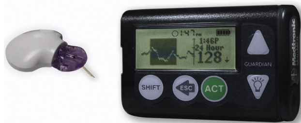
Figure 1 Continuous glucose monitoring system Medtronic Guardian® RT.
