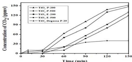
Figure 4 CO<sub>2</sub> selectivity in the acetaldehyde decomposition by TiO<sub>2</sub> nanoparticles
