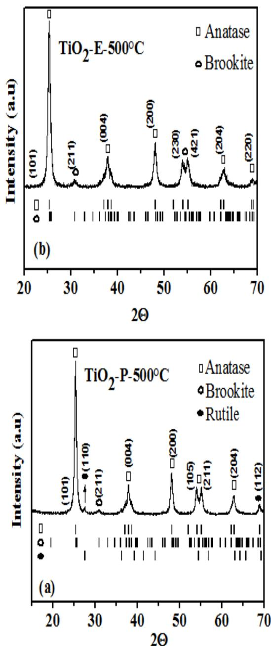
**Figure 1** XRD patterns of the (a)  $\text{TiO}_2\text{-P-500}^\circ\text{C}$  and (b)  $\text{TiO}_2\text{-E-500}^\circ\text{C}$  nanoparticles.
