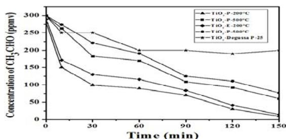
Figure 3. Acetaldehyde conversion as a function of time for the TiO<sub>2</sub> nanoparticles
