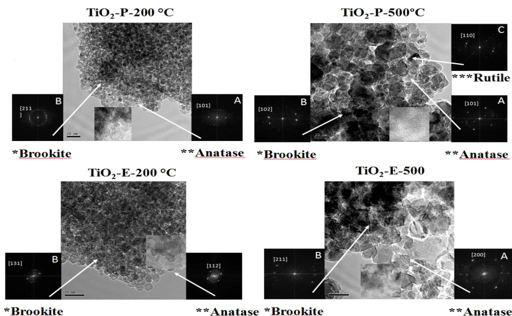
Figure 2 TEM micrographs showing the mixture of the anatase-brookite-rutile phases in the sol-gel TiO<sub>2</sub> nanoparticles
