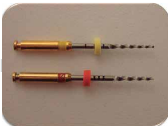
Figure 2. The two fractured instruments: ProTaper Finishing Files F1 (upper) and F2 (lower).
