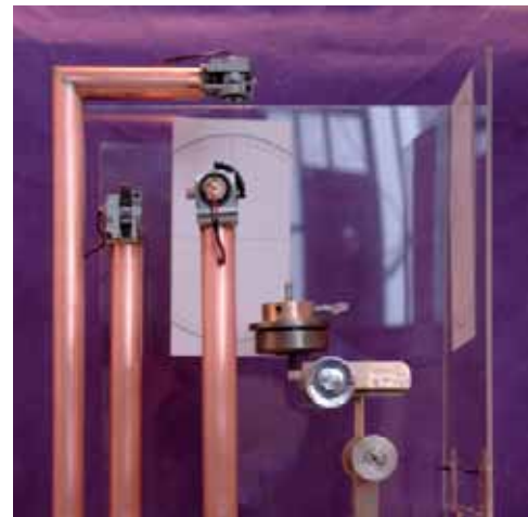
Figure 1. Appliance used for dental surface measurement with the aid of goniometers and laser beam (Patent 264310).
